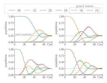
Fig. 5. Evolution of state populations when applying the  $H_4$  pulse of shortest duration (76 ns) to a qudit with d = 4. Every computational basis state is transformed into superposition of all four basis states with nearly equal population, deviations only arising from the remaining 0.1% infidelity. At all times the populations of the guard states  $|4\rangle$  and  $|5\rangle$  are below  $2 \times 10^{-3}$  and  $10^{-6}$ , respectively.
