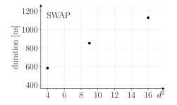
Fig. 8. Gate durations of two-qudit SWAP operations for qudit dimensions d = 2, 3, 4. The x-axis corresponds to the dimension of the full Hilbert space,  $h = d^2$ . Due to the low number of data points, regression is not applied, but a near-linear trend is visible.
