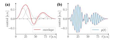
Fig. 2. Real part of an exemplary pulse in the rotating frame, with one carrier wave ( $N_f = 1$ ). (a) Six B-splines shape the envelope of the pulse. Grey dots mark the support of each time-local basis function. (b) The final pulse is constructed from a single carrier wave bounded by the B-spline envelope. With  $N_f > 1$ , the final pulse is the sum of these individual pulses with one carrier wave.
